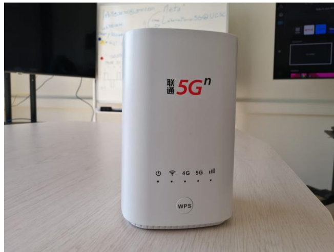
Figura 2.3.4. CPE (Customer Premises Equipment). Fuente: Lab 5G UCSC
