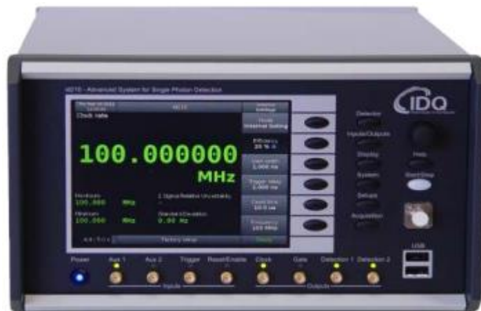
Fig. 2.2 Single Photon Detector ID210 [16]
