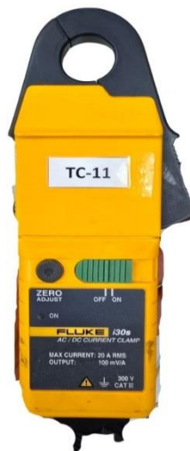
Fig. 7.1 Pinza Amperimetrica CA/CC Fluke I30s.
