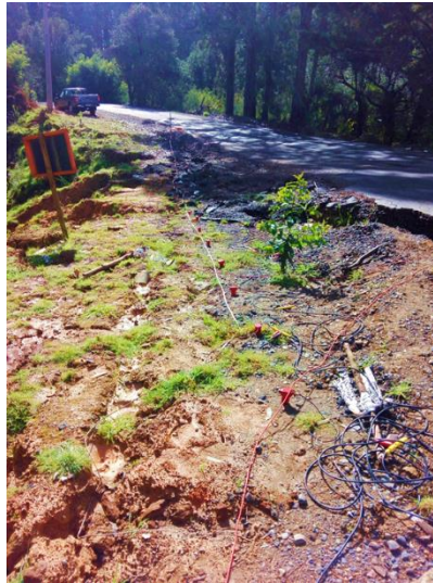
Figure 15: Latitudinal position of receptors along the embankment crest
